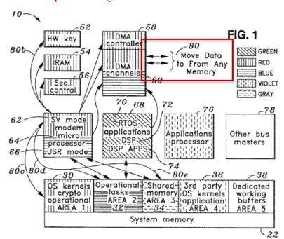
"In another example, a hardware key 52 may be moved in supervisory mode 62 (shown as arrow 80 b) to areas 1, 2 or 3 (shown at 30, 32, and 34 respectively) of system memory 22 as depicted by arrows 80 c, 80 d, and 80 e, respectively. In this particular embodiment, as shown in the foregoing example, **components of a certain level of trust may access memory layers having the same level of trust** or lower (less trusted zones)." *Qualcomm* at col. 5:60-67
